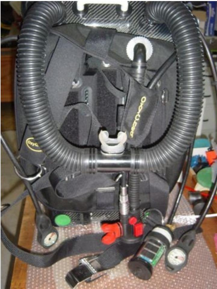
The latest revision of the Abyss rebreather (Nov. 2005). Here we see the front of the unit with revised triple oxygen sensor display lying between the diluent SPG and the OC bailout/ BCD inflator (with red buttons and mouthpiece) on the left hand side of the unit. The SPG for the oxygen cylinder is on the right hand side of the unit. Unlike watching the needle on the SPG of OC equipment, the needles on these SPG's move very slowly indeed!
